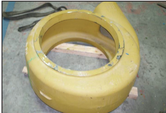
New pump casing before application of ARC
