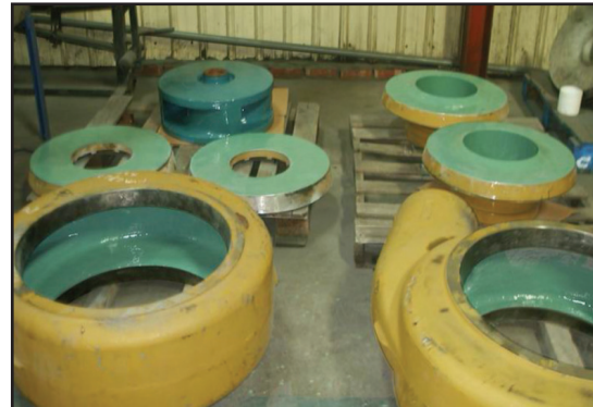
Two new pumps protected with ARC
